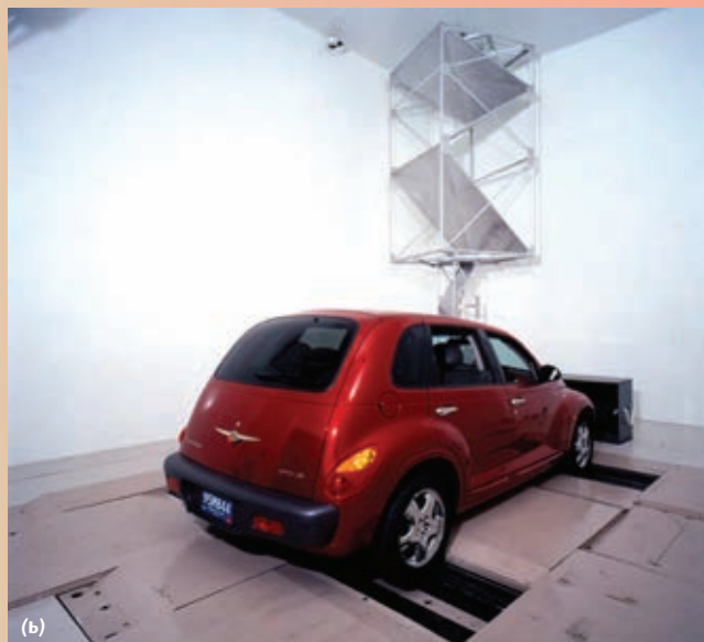
▲ Fig. 5 Component (a) and full vehicle reverb test chambers (b). (Image courtesy of ETS-Lindgren.)
